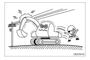
Watch out for obstacles. Be particularly careful to check the machine clearance during the swing.
